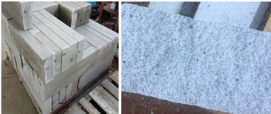
Figure 1. The Cellular Lightweight Concrete (CLC) brick and the texture of CLC brick.
