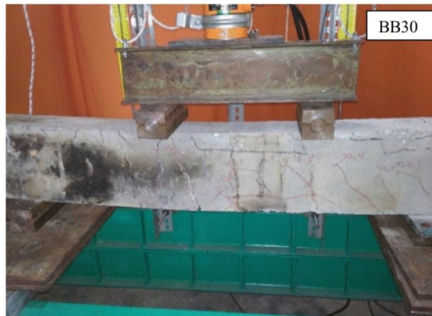
Figure 4. Flexural testing on RC beam BB30 model.
