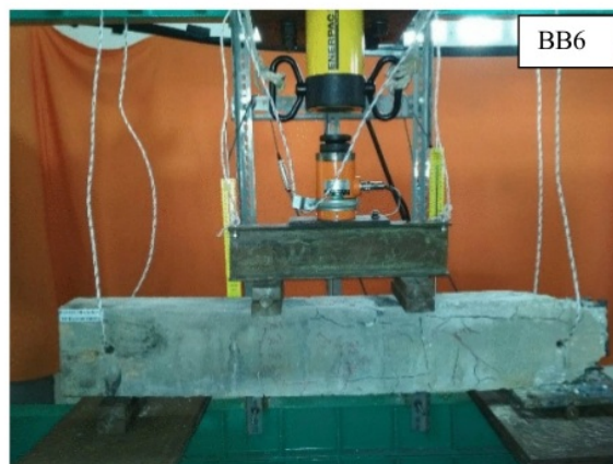
Figure 5. Flexural testing on RC beam BB60 model.
