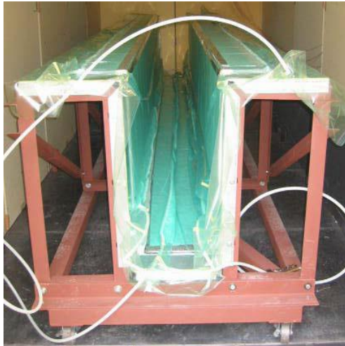
VARTM production of a beam (Robinson, 2008)
