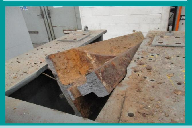
Failure was catastrophic, this fragment weighing about 1.5 tonnes jumped off the test rig. Testing cast iron is dangerous AC IC
