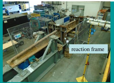
Test rig applied load through jacks at each end. Loads reacted at third points. Set-up not ideal, reaction frames deflected under load and displacement measurement difficult
